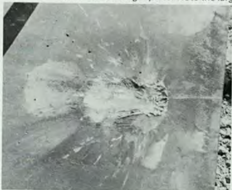
The front and rear of armour plate attacked by 76mm HESH at 45°. Note the size of scab.
