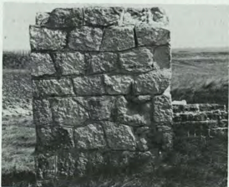
A thick stone wall before and after attack by 76mm HESH.
